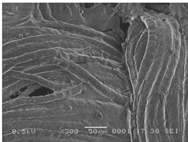
Figure 7 SEM photographs of the woolen fabrics oxidized with potassium permanganate and then cured with CA and chitosan at 120°C for 2 min (300×).
